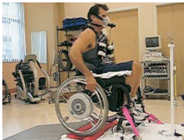
Fig 1. A study participant prepared for metabolic monitoring with the wheelchair secured on stationary rollers and a PAPA mounted on the wheelchair.
